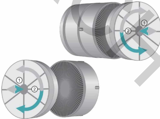
Pic. 14 Carbon filter installation
