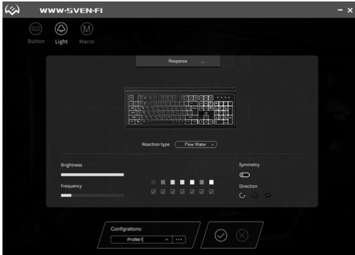
Light menu helps configure the keyboard backlight and includes the following operation modes:
